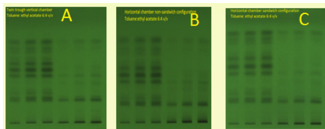
Figure 2: Thin-layer chromatographic separation of Piper guineense seed and leaf extracts with the optimum solvent combination toluene-ethyl acetate (6:4) in an unsaturated twin-trough chamber (A), horizontal developing chamber in nonsandwich configuration (B) and horizontal developing chamber in sandwich configuration (C).
