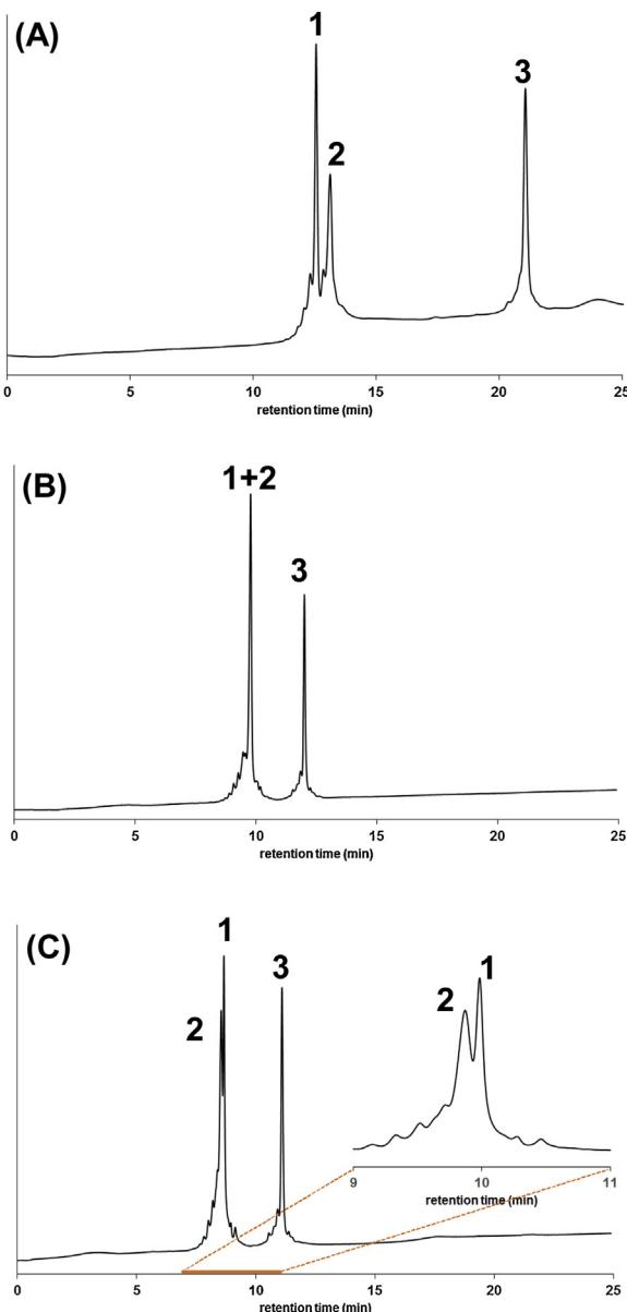
**Fig. 4.** Illustration of the effect of salt concentration on selectivity and elution order of intact mAbs. Column: YMC BioPro SP-F (100 × 4.6 mm, 5 µm), flow rate: 0.8 ml/min, generic gradient: 0–100% in 24 min, temperature: 25 °C, salt concentration:  $c_{s1} = 20$  mM (A),  $c_{s2} = 60$  mM (B) and  $c_{s3} = 100$  mM (C). Peaks: daratumumab (1), obinutuzumab (2) and rituximab (3).
