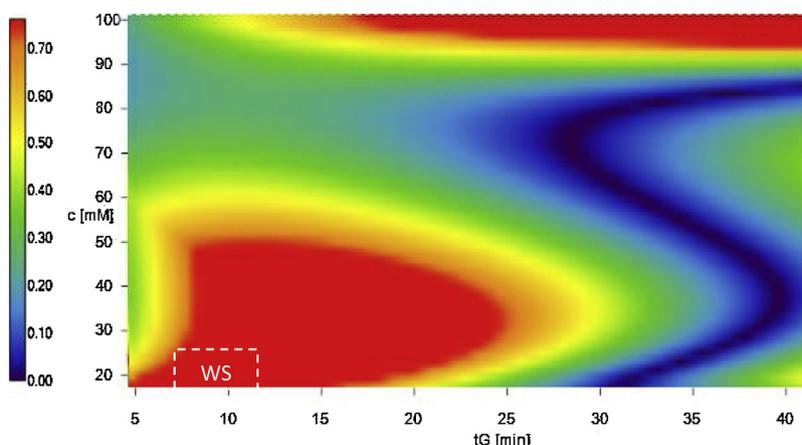
**Fig. 7.** Two dimensional, resolution map ( $tG \times c_s$ ) obtained for cetuximab, subunit separation. Column: YMC BioPro SP-F ( $100 \times 4.6$  mm,  $5 \mu\text{m}$ ), flow rate: 0.8 ml/min, mobile phase system: MES/DAP pH gradient + NaCl salt gradient, temperature:  $25^\circ\text{C}$ , injected volume:  $2 \mu\text{l}$ , detection: FL (280–350 nm).
