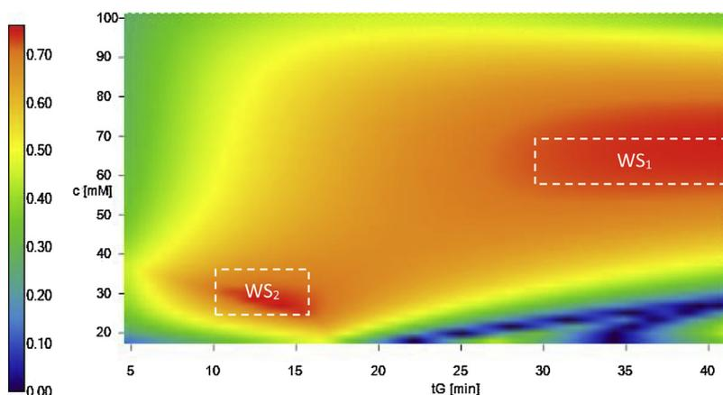
**Fig. 5.** Two dimensional, resolution map ( $tG \times c_s$ ) obtained for daratumumab subunit separation. Column: YMC BioPro SP-F ( $100 \times 4.6$  mm,  $5 \mu\text{m}$ ), flow rate: 0.8 ml/min, mobile phase system: MES/DAP pH gradient + NaCl salt gradient, temperature:  $25^\circ\text{C}$ , injected volume:  $1 \mu\text{l}$ , detection: FL (280–350 nm). Promising working spaces (WS) were indicated as  $WS_1$  and  $WS_2$  (corresponds to optimal conditions).
