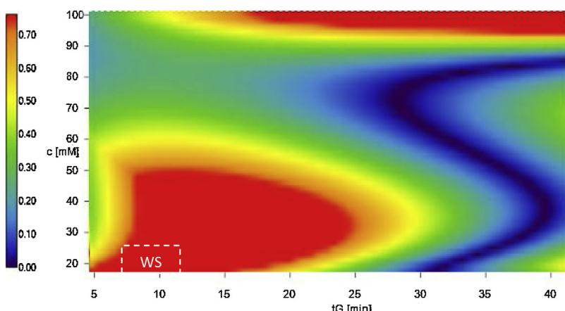
**Fig. 7.** Two dimensional, resolution map ( $t_G \times c_s$ ) obtained for cetuximab, subunit separation. Column: YMC BioPro SP-F (100 × 4.6 mm, 5  $\mu\text{m}$ ), flow rate: 0.8 ml/min, mobile phase system: MES/DAP pH gradient + NaCl salt gradient, temperature: 25 °C, injected volume: 2  $\mu\text{l}$ , detection: FL (280–350 nm).
