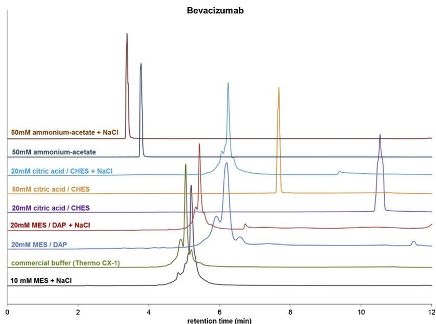
**Fig. 2.** Cation-exchange chromatograms of intact bevacizumab (1 mg/ml) obtained with various buffer systems. Column: YMC BioPro SP-F (100 × 4.6 mm, 5 μm), flow rate: 0.8 ml/min, generic gradient: 0–100% B in 10 min, temperature: 25 °C, injected volume: 1 μl, detection: FL (280–350 nm).
