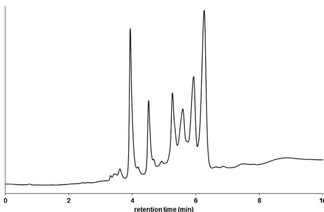
**Fig. 8.** Experimental chromatogram of digested cetuximab, obtained under optimized conditions. Column: YMC BioPro SP-F ( $100 \times 4.6$  mm,  $5 \mu\text{m}$ ), flow rate:  $0.8 \text{ mL/min}$ , mobile phase A: 90%  $20 \text{ mM MES} + 10\% 20 \text{ mM DAP}$ , mobile phase B: 30%  $20 \text{ mM MES} + 70\% 20 \text{ mM DAP} + 20 \text{ mM NaCl}$ . Gradient program: 15–70% B in 8 min, temperature:  $25^\circ\text{C}$ , injected volume:  $2 \mu\text{L}$ , detection: FL (280–350 nm).
