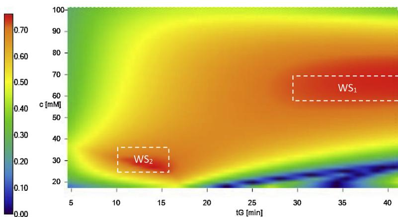
**Fig. 5.** Two dimensional, resolution map ( $t_G \times c_s$ ) obtained for daratumumab subunit separation. Column: YMC BioPro SP-F (100 × 4.6 mm, 5  $\mu\text{m}$ ), flow rate: 0.8 ml/min, mobile phase system: MES/DAP pH gradient + NaCl salt gradient, temperature: 25 °C, injected volume: 1  $\mu\text{l}$ , detection: FL (280–350 nm). Promising working spaces (WS) were indicated as WS<sub>1</sub> and WS<sub>2</sub> (corresponds to optimal conditions).
