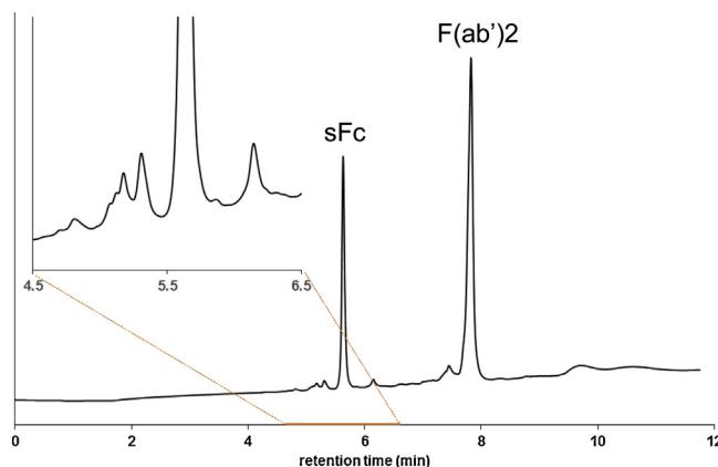
**Fig. 6.** Experimental chromatogram of digested daratumumab, obtained under optimized conditions (corresponding to WS<sub>2</sub>, conditions as specified in Fig. 7 C). Mobile phase A: 90% 20 mM MES + 10% 20 mM DAP, mobile phase B: 30% 20 mM MES + 70% 20 mM DAP + 30 mM NaCl.
