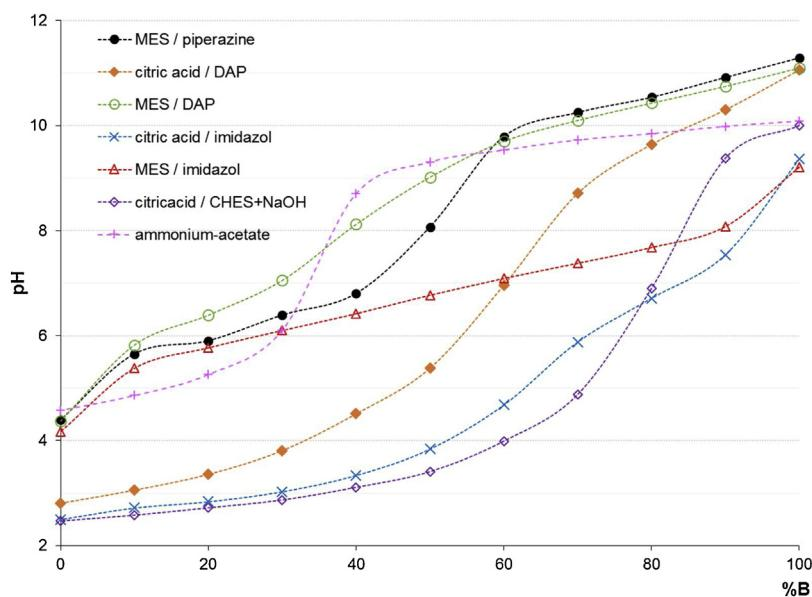
**Fig. 1.** Measured pH responses of various buffer systems as a function of base content.
