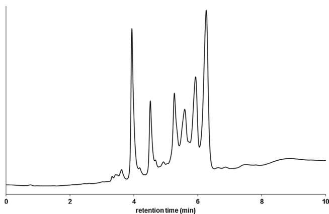
**Fig. 8.** Experimental chromatogram of digested cetuximab, obtained under optimized conditions. Column: YMC BioPro SP-F (100 × 4.6 mm, 5 μm), flow rate: 0.8 ml/min, mobile phase A: 90% 20 mM MES + 10% 20 mM DAP, mobile phase B: 30% 20 mM MES + 70% 20 mM DAP + 20 mM NaCl. Gradient program: 15–70% B in 8 min, temperature: 25 °C, injected volume: 2 μl, detection: FL (280–350 nm).
