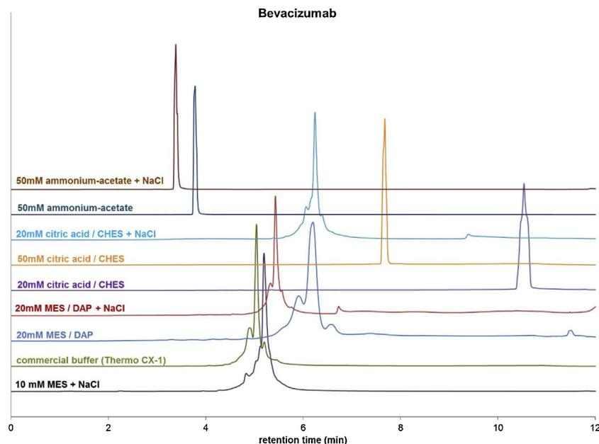
**Fig. 2.** Cation-exchange chromatograms of intact bevacizumab (1 mg/ml) obtained with various buffer systems. Column: YMC BioPro SP-F (100 × 4.6 mm, 5 µm), flow rate: 0.8 ml/min, generic gradient: 0–100% B in 10 min, temperature: 25 °C, injected volume: 1 µl, detection: FL (280–350 nm).
