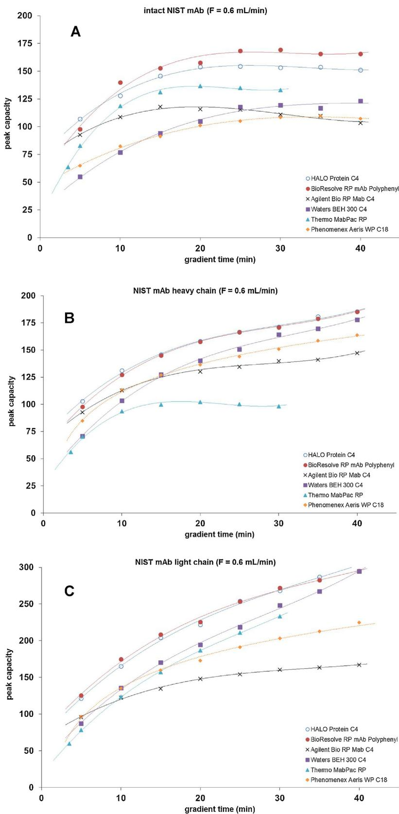
**Fig. 1.** Peak capacity versus gradient time plots of intact NIST mAb (A) and its heavy- (B) and light chains (C) observed at a flow rate of 0.6 mL/min, temperature of 80 °C and with  $\Delta\phi = 0.15$ .
