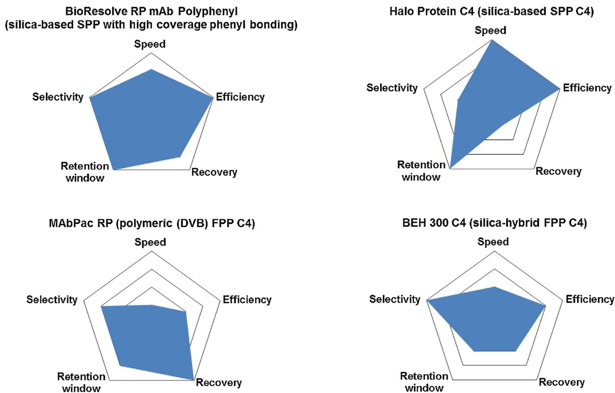
**Fig. 8.** Spidergram representation of the features of the different wide-pore columns based on selectivity, retention window, recovery, efficiency (peak capacity) and separation speed (permeability  $\times$  operating pressure capability).
