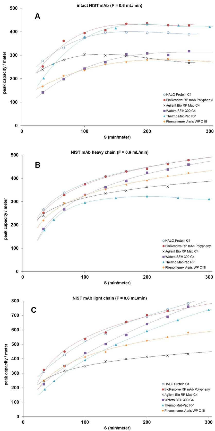
**Fig. 2.** Peak capacity versus gradient steepness plots related to 1 m column length of intact NIST mAb (A) and its heavy- (B) and light chains (C) observed at a flow rate of 0.6 mL/min, temperature of 80 °C and with  $\Delta\Phi = 0.15$ .
