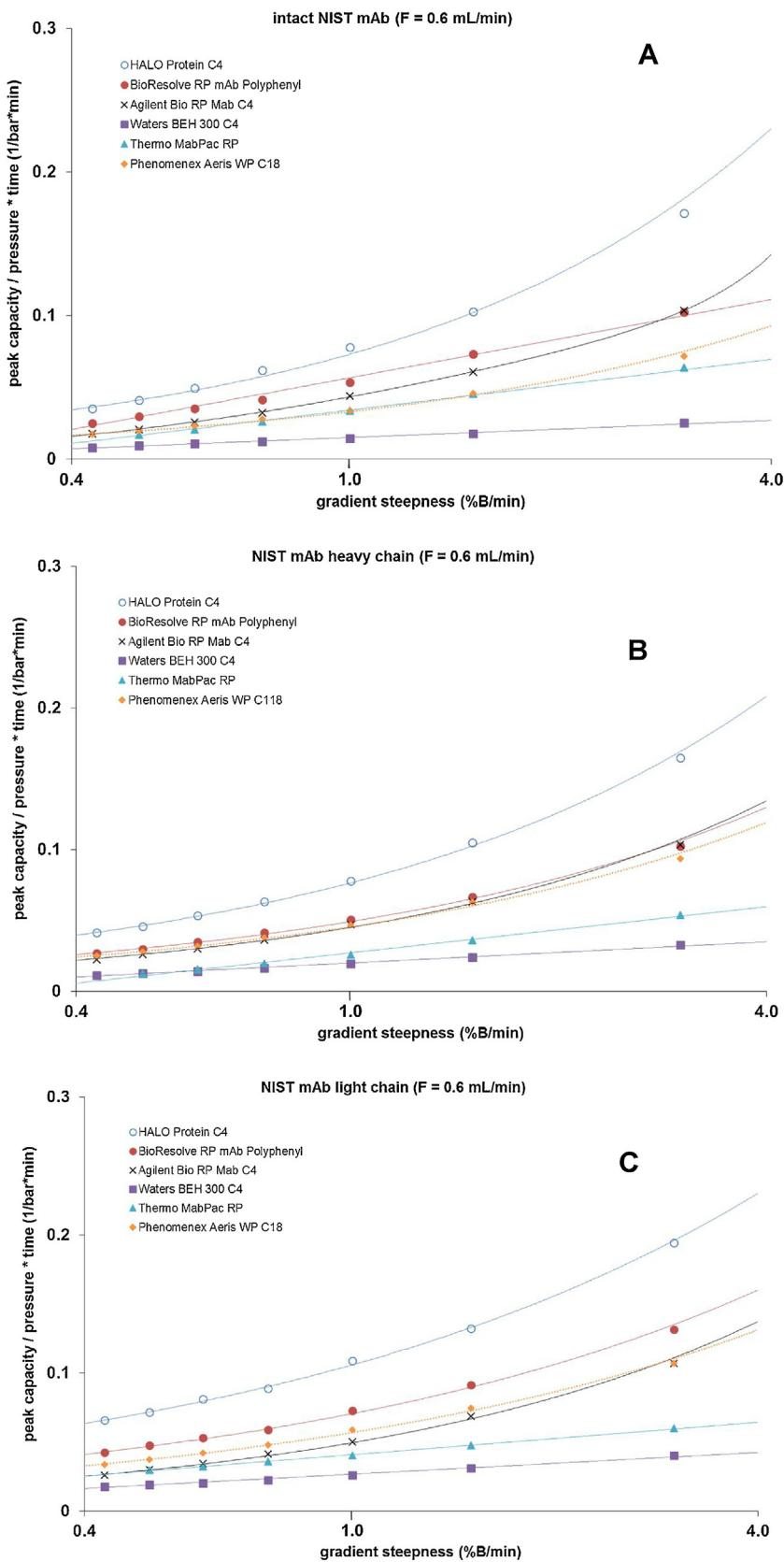
**Fig. 3.** Peak capacity per pressure and time unit versus gradient steepness plots of intact NIST mAb (A) and its heavy- (B) and light chain (C) observed at a flow rate of 0.6 mL/min, temperature of 80 °C and with  $\Delta\phi = 0.15$ .
