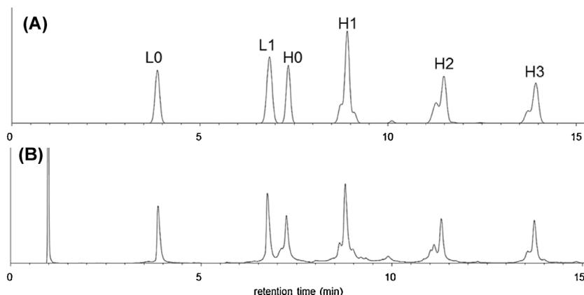
**Fig. 8.** Predicted (A) and experimentally verified (B) chromatograms of reduced Brentuximab vedotin under optimal conditions to optimize resolution between L1 and H0 species. Gradient: 31–48% B,  $t_G = 18$  min,  $T = 90$  °C and  $tC = 20\%$  MeOH (80% AcN). (Column: Agilent Advance BioMAb RP C4, flow rate: 0.3 mL/min).
