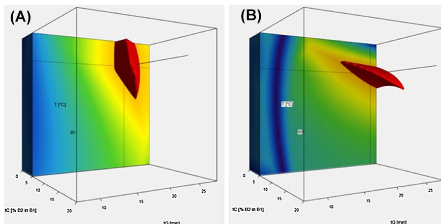
**Fig. 6.** 3D resolution maps for Brentuximab vadotin (A) and for Brentuximab vedotin reduced (B) samples, based on the initial experiments ( $R_s \text{ crit} = 1.0$ ). Set conditions for the native sample:  $t_G = 23$  min,  $T = 88$  °C and  $tC = 5\%$  MeOH. Set conditions for the reduced sample:  $t_G = 27$  min,  $T = 87$  °C and  $tC = 5\%$  MeOH. (For interpretation of the references to colour in the text, the reader is referred to the web version of this article.)
