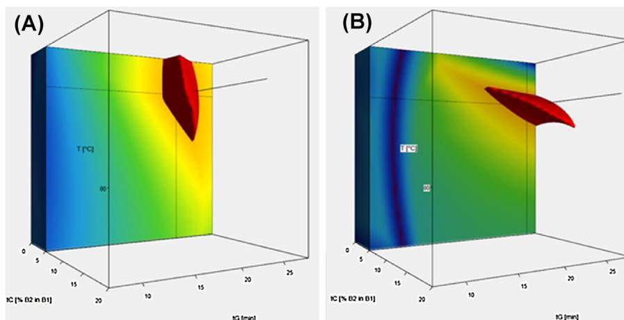
**Fig. 6.** 3D resolution maps for Brentuximab vadotin (A) and for Brentuximab vedotin reduced (B) samples, based on the initial experiments ( $R_s$  crit = 1.0). Set conditions for the native sample:  $t_R = 23$  min,  $T = 88^\circ\text{C}$  and  $t_C = 5\%$  MeOH. Set conditions for the reduced sample:  $t_R = 27$  min,  $T = 87^\circ\text{C}$  and  $t_C = 5\%$  MeOH. (For interpretation of the references to colour in the text, the reader is referred to the web version of this article.)
