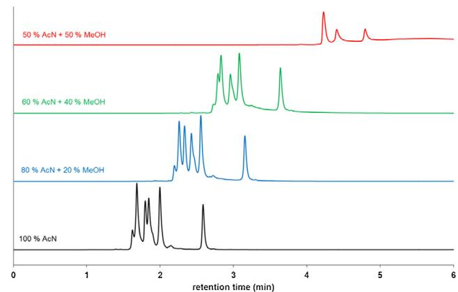
**Fig. 3.** The impact of mobile phase ternary composition. Column: Agilent Advance BioMAB RP C4. Mobile phase "A": 0.1% TFA in water, "B": 0.1% TFA in acetonitrile and methanol mixture. Flow rate: 0.3 mL/min, gradient: 30–80% B in 6 min (extended gradient to enable eluting all the peaks with 50% MeOH content), temperature: 90°C, injected volume: 1 μL, detection at 280 nm. Sample: Brentuximab vedotin.
