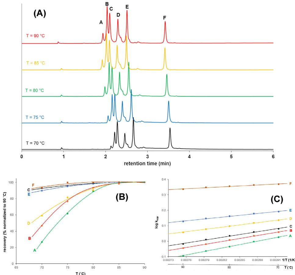
**Fig. 2.** The impact of mobile phase temperature on the retention times (A), peak area (recovery) (B) and retention factor (C) of different ADC species. Column: Agilent Advance BioMAb RP C4. Mobile phase “A”: 0.1% TFA in water, “B”: 0.1% TFA in acetonitrile. Flow rate: 0.3 mL/min, gradient: 30–60% B in 6 min (extended gradient to enable baseline resolution and the measurement of peak areas), temperature: 90 °C, injected volume: 1 μL, detection at 280 nm. Sample: Brentuximab vedotin.
