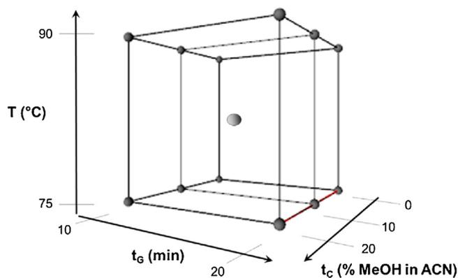
**Fig. 4.** Suggested experimental design for 3D retention model (column: 150 × 2.1 mm, gradient: 25–50% B at 0.3 mL/min).
