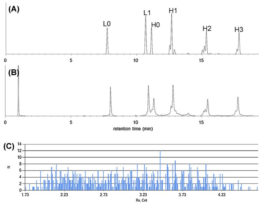
**Fig. 9.** Predicted (A) and experimentally verified (B) chromatograms of reduced Brentuximab vedotin under optimal conditions to optimize resolution between all peaks. Gradient: 25–50% B,  $t_G=27$  min,  $T=87^\circ\text{C}$  and  $t_C=5\%$  MeOH (95% AcN). (Column: Agilent Advance BioMab RP C4, flow rate: 0.3 mL/min). Panel C represents the result of simulated robustness test as number of observations (N) vs. critical resolution ( $R_{s,crit}$ ).
