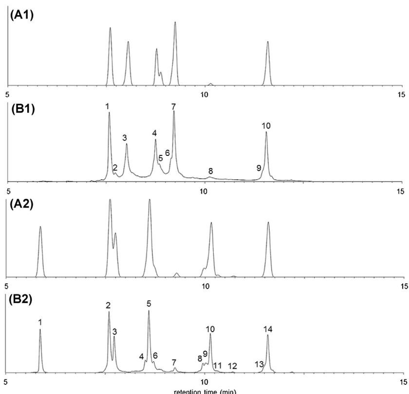
**Fig. 5.** Model verification in the center point for native Brentuximab vedotin (1) and for reduced Brentuximab vedotin (2). Column: Agilent Advance BioMAb RP C4. Mobile phase "A": 0.1% TFA in water, "B": 0.1% TFA in 90% acetonitrile + 10% MeOH. Flow rate: 0.3 mL/min, gradient: 25–50% B in 15 min, temperature: 82.5 °C, injected volume: 1 μL, detection at 280 nm. "A" corresponds to predicted, while "B" corresponds to experimental chromatograms.
