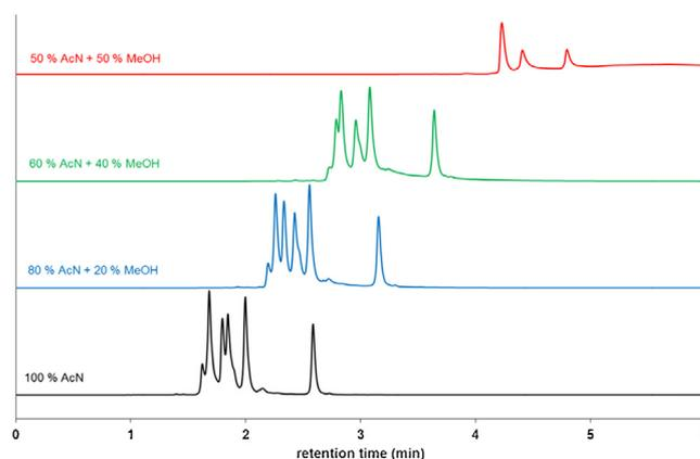
**Fig. 3.** The impact of mobile phase ternary composition. Column: Agilent Advance BioMab RP C4. Mobile phase "A": 0.1% TFA in water, "B": 0.1% TFA in acetonitrile and methanol mixture. Flow rate: 0.3 mL/min, gradient: 30–80% B in 6 min (extended gradient to enable eluting all the peaks with 50% MeOH content), temperature:  $90^\circ\text{C}$ , injected volume: 1  $\mu\text{L}$ , detection at 280 nm. Sample: Brentuximab vedotin.
