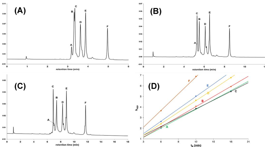
**Fig. 1.** The impact of gradient steepness on selectivity. Column: Agilent Advance BioMAb RP C4. Mobile phase “A”: 0.1% TFA in water, “B”: 0.1% TFA in acetonitrile. Flow rate: 0.3 mL/min, gradient: 25–50% B (in 6 min (A), 12 min (B) and 18 min (C)), temperature: 90 °C, injected volume: 1 μL, detection at 280 nm. Panel D shows the dependence of  $k_{app}$  on the gradient time. Sample: Brentuximab vedotin.
