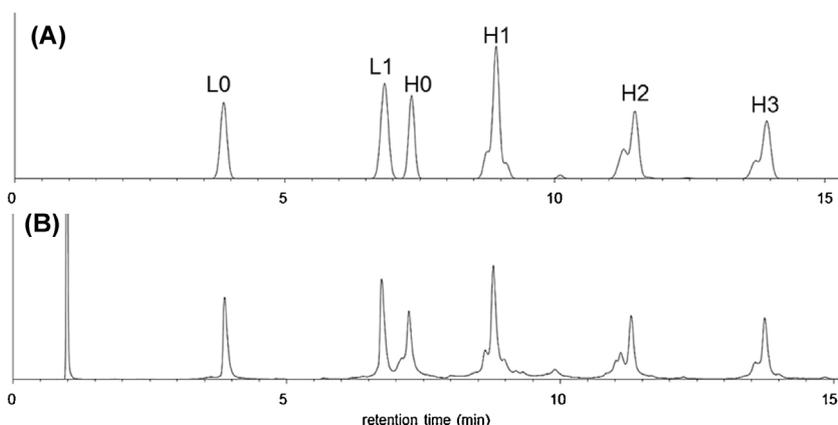
**Fig. 8.** Predicted (A) and experimentally verified (B) chromatograms of reduced Brentuximab vedotin under optimal conditions to optimize resolution between L1 and H0 species. Gradient: 31–48% B,  $t_C = 18$  min,  $T = 90^\circ\text{C}$  and  $t_C = 20\%$  MeOH (80% AcN). (Column: Agilent Advance BioMAB RP C4, flow rate: 0.3 mL/min).
