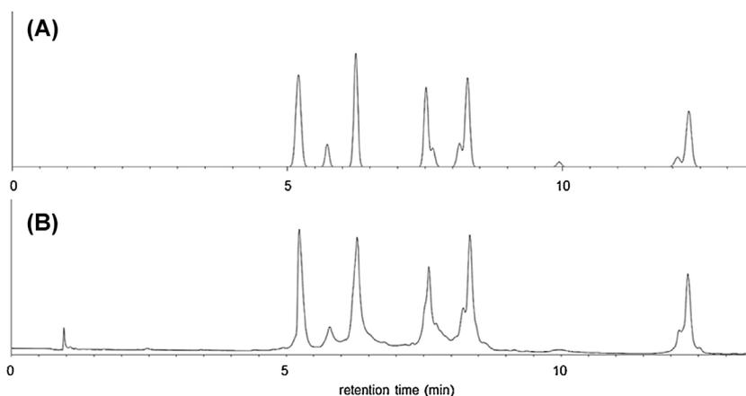
**Fig. 7.** Predicted (A) and experimentally verified (B) chromatograms of native Brentuximab vedotin under optimal conditions. Gradient: 29–42% B,  $t_C = 14$  min,  $T = 90^\circ\text{C}$  and  $t_C = 0\%$  MeOH (100% AcN). (Column: Agilent Advance BioMAB RP C4, flow rate: 0.3 mL/min).
