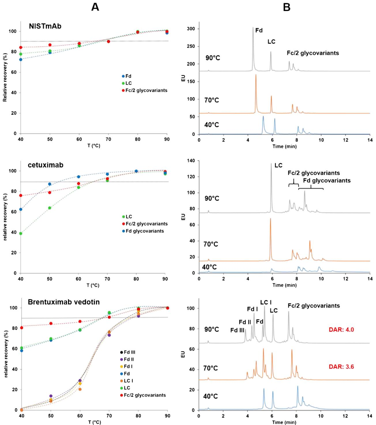
**Fig. 3.** (A) Relative recovery of NISTmAb, cetuximab and brentuximab vedotin subunits as a function of mobile phase temperature. (B) Corresponding chromatograms at 40 °C, 70 °C and 90 °C. Gradient: 75–60%B in 15 min. A: H<sub>2</sub>O + 0.1% TFA, B: ACN + 0.1% TFA. Flow: 0.45 mL/min. Column: Waters Acquity UPLC Glycoprotein BEH Amide (300 Å, 1.7 μm, 2.1 mm × 150 mm).
