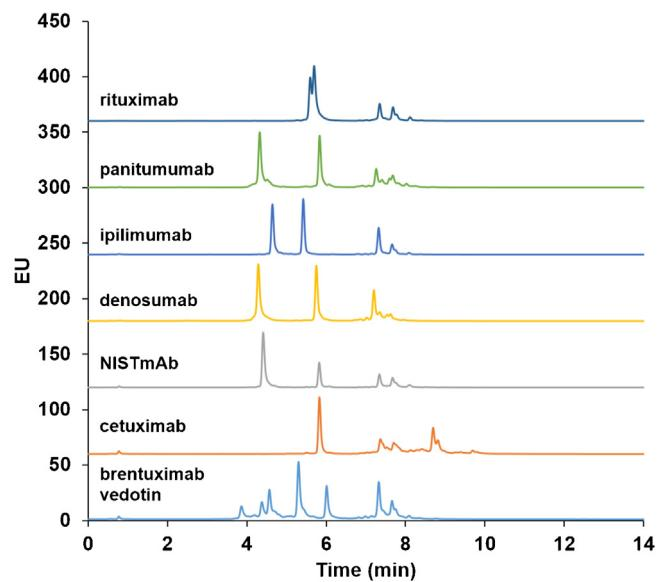
**Fig. 2.** General HILIC chromatograms of IdeS digested and reduced mAb and ADC samples. Gradient: 75–60% B in 15 min. A:  $\text{H}_2\text{O} + 0.1\%$  TFA, B ACN + 0.1% TFA. T: 80 °C, flow: 0.45 mL/min. Column: Waters Acuity UPLC Glycoprotein BEH Amide (300 Å, 1.7 μm, 2.1 mm × 150 mm).
