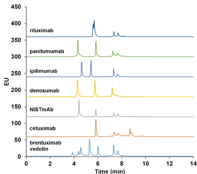
**Fig. 2.** General HILIC chromatograms of IdeS digested and reduced mAb and ADC samples. Gradient: 75–60%B in 15 min. A: H<sub>2</sub>O + 0.1% TFA, B ACN + 0.1% TFA. T: 80 °C, flow: 0.45 mL/min. Column: Waters Acquity UPLC Glycoprotein BEH Amide (300 Å, 1.7 μm, 2.1 mm × 150 mm).
