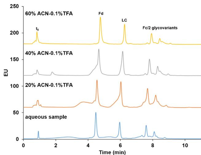
**Fig. 1.** HILIC chromatograms of IdeS digested and reduced trastuzumab when injecting from different sample solvents and using linear gradient without initial fast gradient ramp. Gradient: 74–68%B in 15 min. A: H<sub>2</sub>O + 0.1% TFA, B ACN + 0.1% TFA. Other chromatographic conditions are detailed in Section 2.3.
