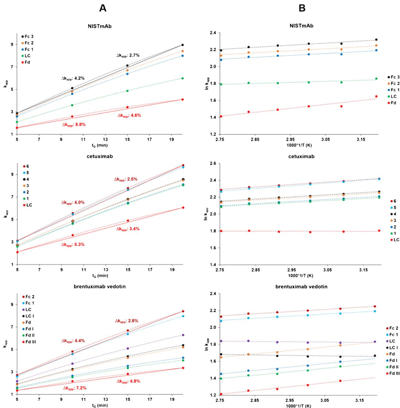
**Fig. 4.** (A) Retention as a function of gradient time, (B) Van't Hoff plots of NISTmAb, cetuximab and brentuximab vedotin subunits. Gradient: 75–60% B. A: H<sub>2</sub>O + 0.1% TFA, B: ACN + 0.1% TFA, flow: 0.45 mL/min. Column: Waters Acquity UPLC Glycoprotein BEH Amide (300 Å, 1.7 μm, 2.1 mm × 150 mm). Other chromatographic conditions are detailed in Section 3.3.
