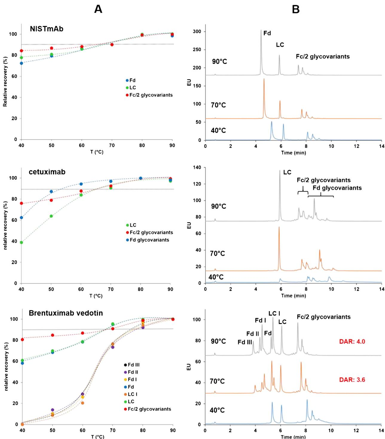
**Fig. 3.** (A) Relative recovery of NISTmAb, cetuximab and brentuximab vedotin subunits as a function of mobile phase temperature. (B) Corresponding chromatograms at 40 °C, 70 °C and 90 °C. Gradient: 75–60% B in 15 min. A: H<sub>2</sub>O + 0.1% TFA, B: ACN + 0.1% TFA. Flow: 0.45 mL/min. Column: Waters Acuity UPLC Glycoprotein BEH Amide (300 Å, 1.7 µm, 2.1 mm × 150 mm).
