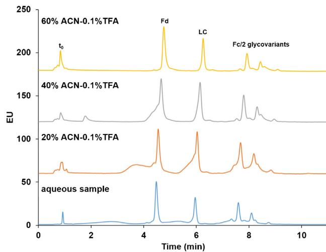
**Fig. 1.** HILIC chromatograms of IdeS digested and reduced trastuzumab when injecting from different sample solvents and using linear gradient without initial fast gradient ramp. Gradient: 74–68% B in 15 min. A:  $\text{H}_2\text{O} + 0.1\%$  TFA, B ACN + 0.1% TFA. Other chromatographic conditions are detailed in Section 2.3.
