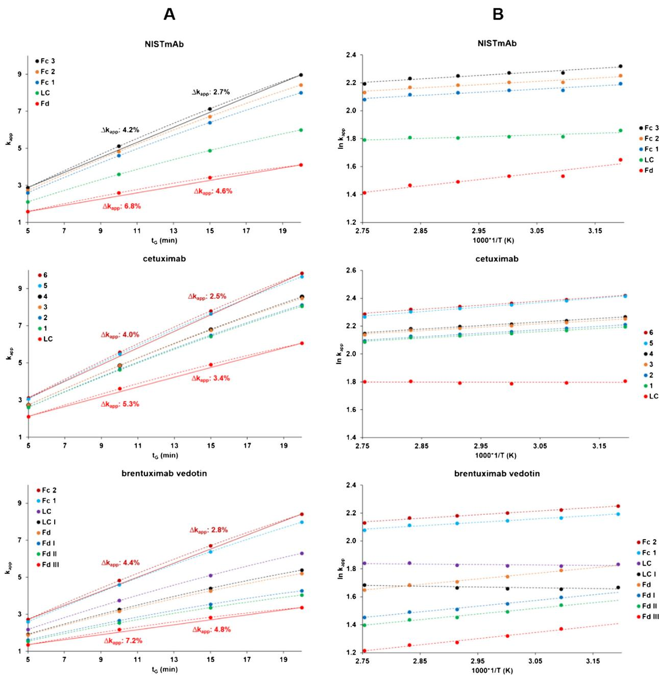
**Fig. 4.** (A) Retention as a function of gradient time, (B) Van't Hoff plots of NISTmAb, cetuximab and brentuximab vedotin subunits. Gradient: 75–60%B. A: H<sub>2</sub>O+0.1% TFA, B: ACN+0.1% TFA, flow: 0.45 mL/min. Column: Waters Acquity UPLC Glycoprotein BEH Amide (300 Å, 1.7  $\mu$ m, 2.1 mm  $\times$  150 mm). Other chromatographic conditions are detailed in Section 3.3.
