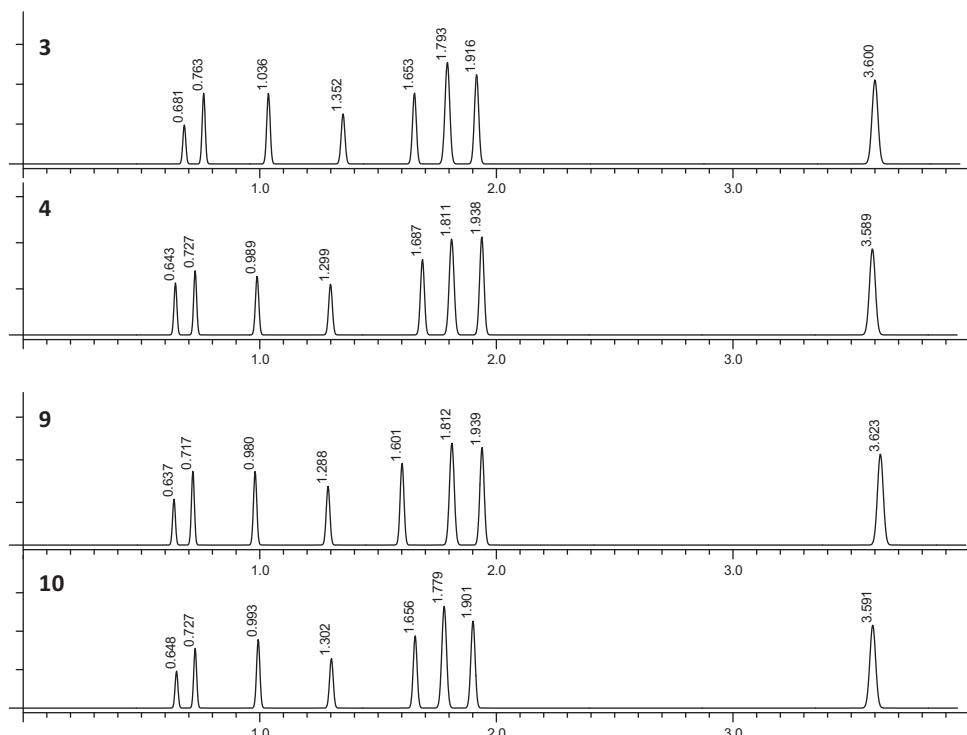
**Fig. 7.** The chromatograms of the identical batches (3–4 and 9–10) at the working point of the highest critical resolution.
