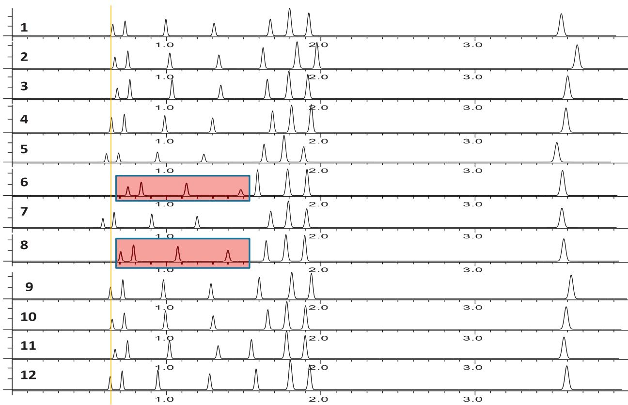
**Fig. 6.** Chromatograms of the highest resolution of each column. The retention order is impurities D, F, amlodipine, impurities E, H, G, B, A. Basic compounds (red boxes) are retarded more in the columns no. 6 and 8. The critical resolution however is sufficient with all columns. (For interpretation of the references to color in this figure legend, the reader is referred to the web version of this article.)
