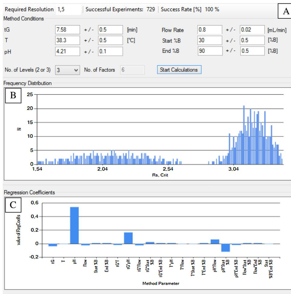
**Fig. 9.** The tolerance limits were changed to the performance values of the instrument (C). Regression coefficients (A) and the frequency distribution of the critical resolution (B) in the 729 virtual experiments of column no. 1 (Batch 154) in the DryLab®4 Robustness Module.
