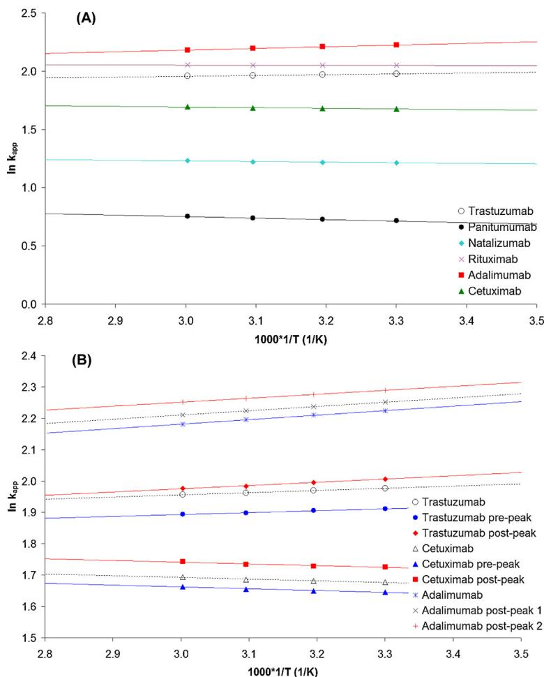
**Fig. 2.** Effect of temperature on the apparent retention factor of native antibodies (A) and antibody variants (B) (van't Hoff type representation). Column: YMC BioPro SP-F (100 × 4.6 mm). Mobile phase: "A", 10 mM MES pH 6.3; "B", 10 mM MES pH 6.3 + 1 M NaCl. Flow rate: 0.6 ml/min; gradient: 0–20% B in 15 min; temperature: 30, 40, 50 and 60 °C; detection: FL (280–360 nm); injected volume: 2 µl.
