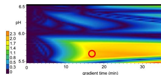
**Fig. 6.** Cetuximab papain digestion resolution map ( $t_g$ -pH model). Column: YMC BioPro SP-F ( $100 \times 4.6$  mm). Mobile phase: "A", 10 mM MES; "B", 10 mM MES + 1 M NaCl. Flow rate: 0.6 ml/min; gradient: 0–20% B; temperature: 30 °C; detection: FL (280–360 nm); injected volume: 2 µl. Gradient times:  $t_{g1} = 10$  min,  $t_{g2} = 30$  min, pH<sub>1</sub> 5.6, pH<sub>2</sub> 6.0, pH<sub>3</sub> 6.4.
