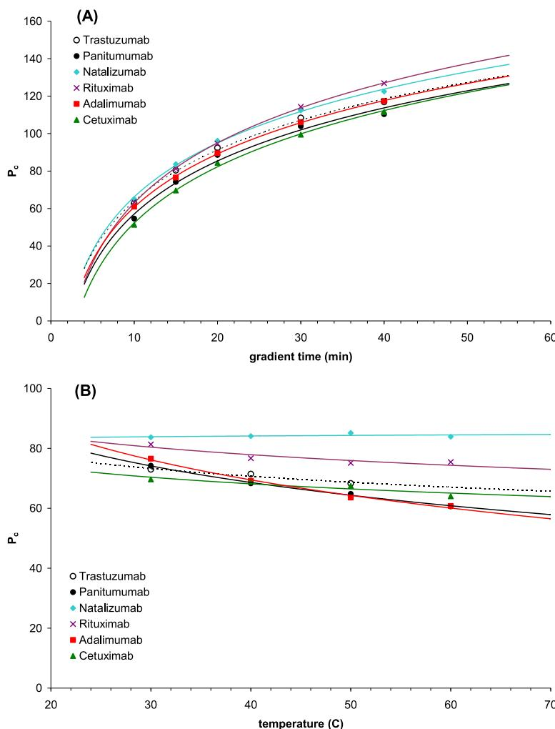
**Fig. 4.** Peak capacity as a function of gradient time (steepness) (A) and temperature (B). Column: YMC BioPro SP-F (100 × 4.6 mm). Mobile phase: "A", 10 mM MES pH 6.3; "B", 10 mM MES pH 6.3 + 1 M NaCl. Flow rate: 0.6 ml/min; detection: FL (280–360 nm); injected volume: 2 µl.
