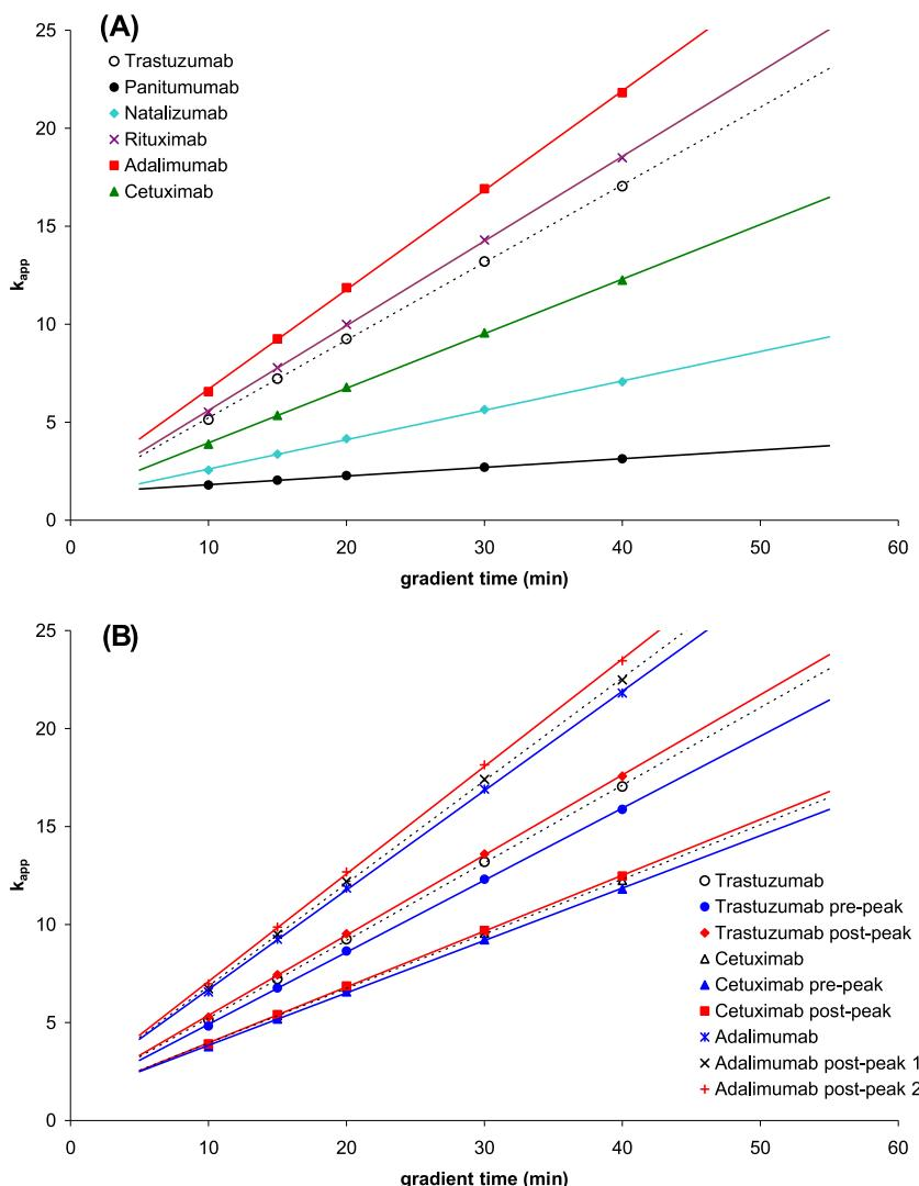
**Fig. 1.** Effect of gradient time (steepness) on the apparent retention factor of native antibodies (A) and antibody variants (B). Column: YMC BioPro SP-F (100 × 4.6 mm). Mobile phase: "A", 10 mM MES pH 6.3; "B", 10 mM MES pH 6.3 + 1 M NaCl. Flow rate: 0.6 ml/min; gradient: 0–20% B in 10, 15, 20, 30 and 40 min; temperature: 30 °C, detection: FL (280–360 nm); injected volume: 2 µl.
