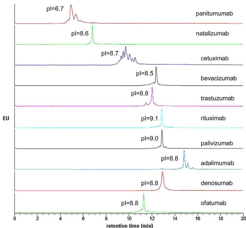
**Fig. 8.** Generic salt gradient. Column: YMC BioPro SP-F (100 × 4.6 mm). Mobile phase: “A”, 10 mM MES pH 5.7; “B”, 10 mM MES pH 5.7 + 1 M NaCl. Flow rate: 0.6 ml/min; gradient: 0–20% B in 20 min; temperature: 30 °C; detection: FL (280–360 nm); injected volume: 2 µl.
