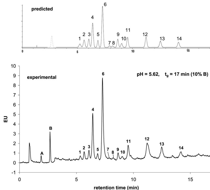
**Fig. 7.** Comparison of predicted and experimental chromatograms. Column: YMC BioPro SP-F ( $100 \times 4.6$  mm). Mobile phase: "A", 10 mM MES; "B", 10 mM MES + 1 M NaCl. Flow rate: 0.6 ml/min; gradient: 0–10% B; temperature: 30 °C; detection: FL (280–360 nm); injected volume: 2 µl. Gradient times:  $t_g = 17$  min, pH 5.62.
