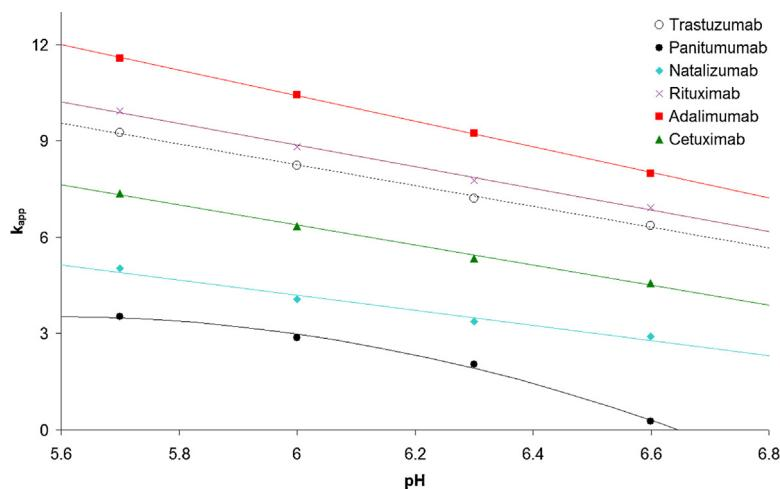
**Fig. 3.** Effect of mobile phase pH on the apparent retention factor of native antibodies. Column: YMC BioPro SP-F (100 × 4.6 mm). Mobile phase: "A", 10 mM MES; "B", 10 mM MES + 1 M NaCl (pH was set at 5.7, 6.0, 6.3 and 6.6). Flow rate: 0.6 ml/min; gradient: 0–20% B in 15 min; temperature: 30 °C; detection: FL (280–360 nm); injected volume: 2 µl.
