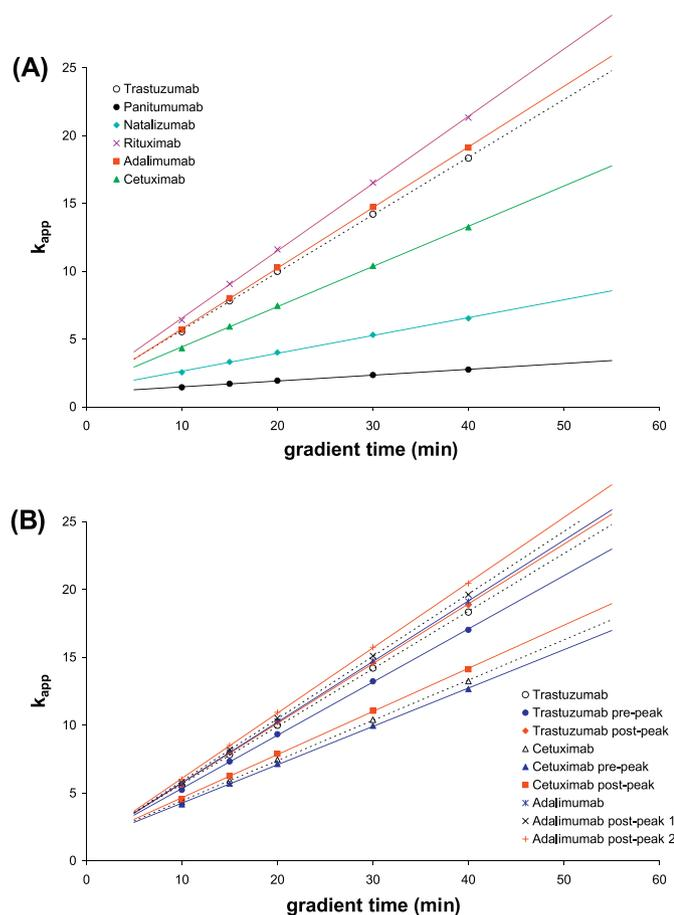
**Fig. 1.** Effect of gradient time (steepness) on the apparent retention factor of native antibodies (A) and antibody variants (B). Column: YMC BioPro SP-F (100 mm × 4.6 mm). Mobile phase “A” CX-1 Buffer A pH 5.6, “B” CX-1 Buffer B pH 10.2. Flow rate: 0.6 ml/min, gradient: 0–100%B in 10, 15, 20, 30 and 40 min, temperature: 30 °C, detection: FL (280–360 nm), injected volume: 2  $\mu$ l.
