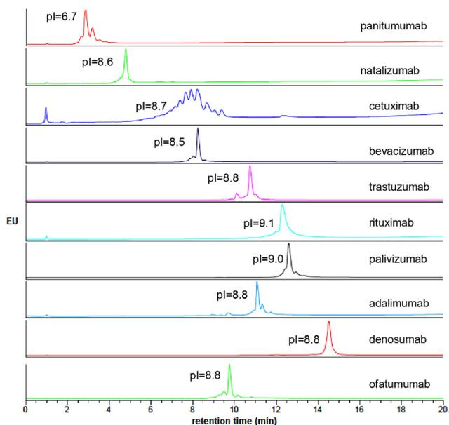
**Fig. 7.** Generic pH gradient. Column: YMC BioPro SP-F (100 mm × 4.6 mm). Mobile phase “A” CX-1 Buffer A pH 5.6, “B” CX-1 Buffer B pH 10.2. Flow rate: 0.6 ml/min, gradient: 0–100%B in 20 min, temperature: 30 °C, detection: FL (280–360 nm), injected volume: 2  $\mu$ l.
