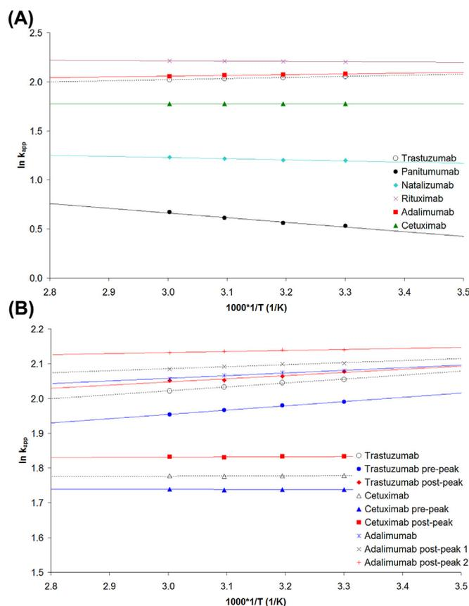
**Fig. 2.** Effect of temperature on the apparent retention factor of native antibodies (A) and antibody variants (B) (van’t Hoff type representation). Column: YMC BioPro SP-F (100 mm × 4.6 mm). Mobile phase “A” CX-1 Buffer A pH 5.6, “B” CX-1 Buffer B pH 10.2. Flow rate: 0.6 ml/min, gradient: 0–100%B in 15 min, temperature: 30, 40, 50 and 60 °C, detection: FL (280–360 nm), injected volume: 2  $\mu$ l.
