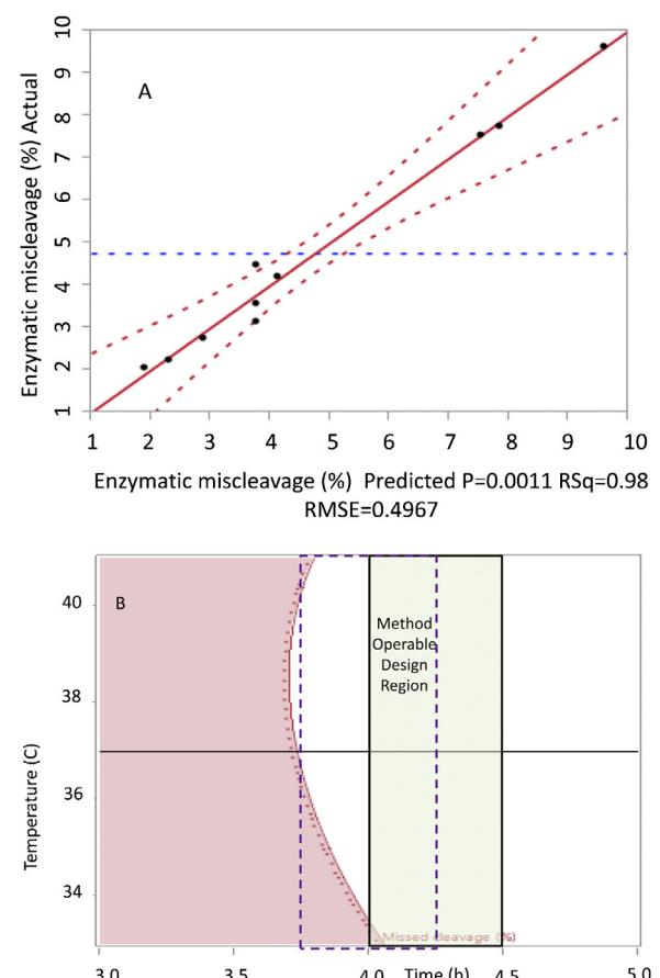
**Fig. 4.** Results from a surface response DOE study, (A) correlation of the predicted with the actual enzymatic miscleavage values and (B) a contour map from the DOE study for digestion time and temperature, the robust method operable design region is shifted from the dashed line rectangle to the solid line rectangle.
