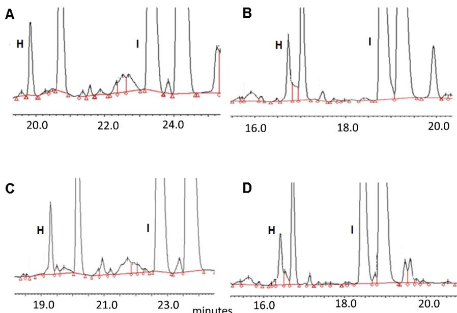
**Fig. 6.** Expanded chromatograms with peaks H and I from the C-terminal heterogeneity assay. All 4HPLC conditions contain 0.09%TFA in mobile phases A (water) and B (acetonitrile). (A) Column temp: 38 °C, ending mobile phase B = 23.7%, (B) column temp: 38 °C, ending mobile phase B = 26.3%, (C) column temp: 42 °C, ending mobile phase B = 23.7% and (D) column temp: 42 °C, ending mobile phase B = 26.3%.
