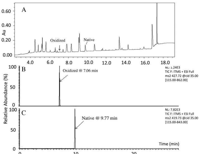
**Fig. 5.** A. A UV chromatogram of a protein digestion. B-C. LC-MS selected ion monitoring chromatograms of an oxidized peptide and its native peptide, respectively.
