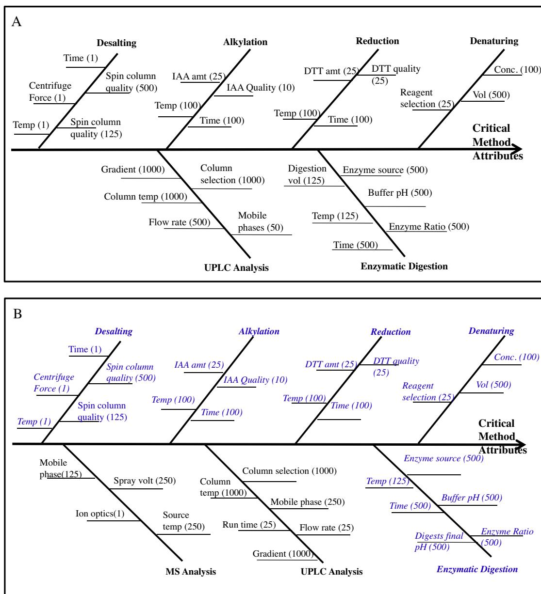
**Fig. 2.** Fishbone diagrams for 2 different methods, (A) peptide map by UHPLC-UV and (B) UHPLC-MS for oxidation analysis.
