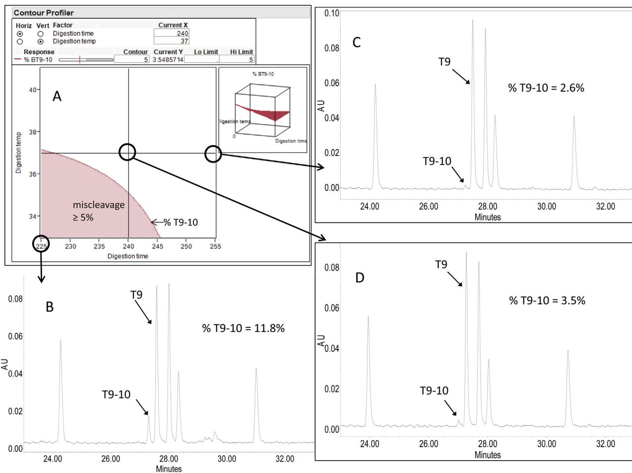
**Fig. 3.** (A) A contour map from the DOE study for enzymatic digestion time and temperature. The acceptable level for T9-10 is  $\leq 5\%$ . (B–D) Chromatograms at different spots on the contour map.
