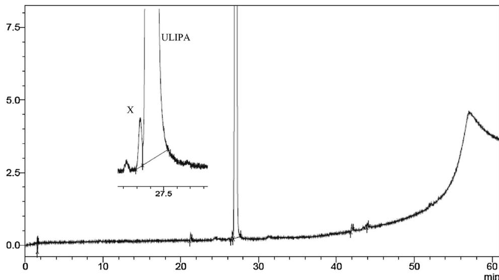
**Fig. 3.** HPLC chromatogram of ulipristal acetate (ULIPA). Kinetex XB-C18 column (150 mm × 4.6 mm, 2.6 µm, Phenomenex, USA); UV detector: 305 nm. Mobile phase A: 990 ml of water + 10 ml of 1 M triethyl ammonium phosphate (TEAP) solution; mobile phase B: 900 ml of acetonitrile + 90 ml of water + 10 ml of TEAP. Gradient program: the ratio of mobile phase B was 25% (0 min), 60% (35 min), 100% (55 min), 100% (60 min). From Ref. [163] with permission.
