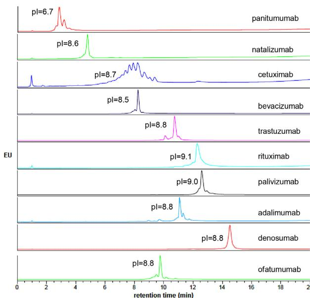
**Fig. 7.** Generic pH gradient. Column: YMC BioPro SP-F (100 mm × 4.6 mm). Mobile phase "A" CX-1 Buffer A pH 5.6, "B" CX-1 Buffer B pH 10.2. Flow rate: 0.6 ml/min, gradient: 0–100% B in 20 min, temperature: 30 °C, detection: FL (280–360 nm), injected volume: 2 µl.
