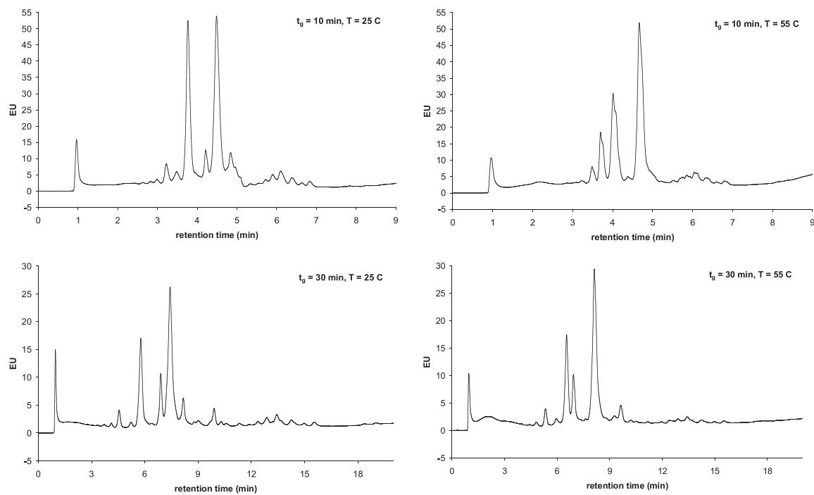
**Fig. 4.** Cetuximab papain digested sample. Column: YMC BioPro SP-F (100 mm × 4.6 mm). Mobile phase "A" CX-1 Buffer A pH 5.6, "B" CX-1 Buffer B pH 10.2. Flow rate: 0.6 ml/min, gradient: 0–80% B, detection: FL (280–360 nm), injected volume: 2 µl. Gradient times:  $t_{g1} = 10$  min,  $t_{g2} = 30$  min, temperatures  $T_1 = 25$  °C,  $T_2 = 55$  °C.
