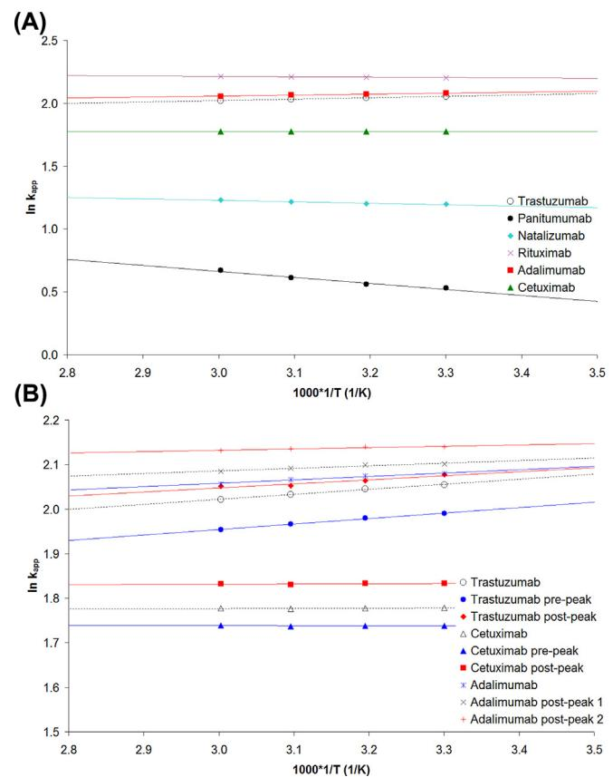
**Fig. 2.** Effect of temperature on the apparent retention factor of native antibodies (A) and antibody variants (B) (van't Hoff type representation). Column: YMC BioPro SP-F (100 mm × 4.6 mm). Mobile phase "A" CX-1 Buffer A pH 5.6, "B" CX-1 Buffer B pH 10.2. Flow rate: 0.6 ml/min, gradient: 0–100% B in 10, 15, 20, 30 and 40 min, temperature: 30, 40, 50 and 60 °C, detection: FL (280–360 nm), injected volume: 2 µl.
