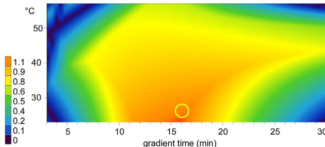
**Fig. 5.** Cetuximab papain digestion resolution map ( $t_g$ -T model). Column: YMC BioPro SP-F (100 mm × 4.6 mm). Mobile phase "A" CX-1 Buffer A pH 5.6, "B" CX-1 Buffer B pH 10.2. Flow rate: 0.6 ml/min, gradient: 0–80% B, detection: FL (280–360 nm), injected volume: 2 µl. Gradient times:  $t_{g1} = 10$  min,  $t_{g2} = 30$  min, temperatures  $T_1 = 25$  °C,  $T_2 = 55$  °C.
