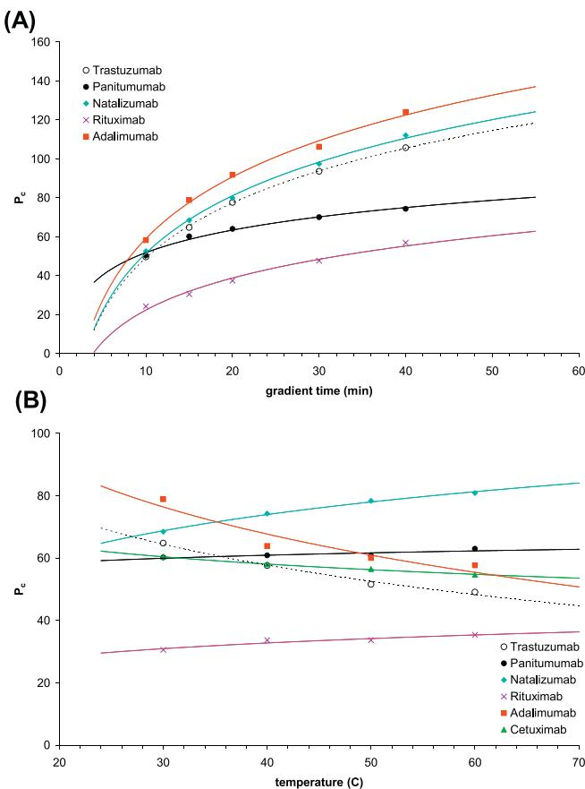
**Fig. 3.** Peak capacity as a function of gradient time (steepness) (A) and temperature (B). Column: YMC BioPro SP-F (100 mm × 4.6 mm). Mobile phase “A” CX-1 Buffer A pH 5.6, “B” CX-1 Buffer B pH 10.2. Flow rate: 0.6 ml/min, detection: FL (280–360 nm), injected volume: 2 µl.
