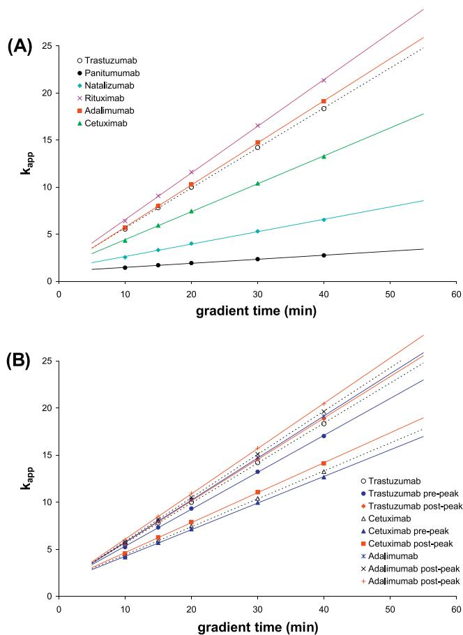
**Fig. 1.** Effect of gradient time (steepness) on the apparent retention factor of native antibodies (A) and antibody variants (B). Column: YMC BioPro SP-F (100 mm × 4.6 mm). Mobile phase "A" CX-1 Buffer A pH 5.6, "B" CX-1 Buffer B pH 10.2. Flow rate: 0.6 ml/min, gradient: 0–100% B in 10, 15, 20, 30 and 40 min, temperature: 30 °C, detection: FL (280–360 nm), injected volume: 2 µl.
