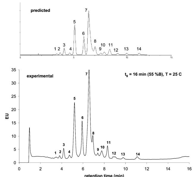
**Fig. 6.** Comparison of predicted and experimental chromatograms. Column: YMC BioPro SP-F (100 mm × 4.6 mm). Mobile phase "A" CX-1 Buffer A pH 5.6, "B" CX-1 Buffer B pH 10.2. Flow rate: 0.6 ml/min, gradient: 0–55% B in 16 min, temperature: 25 °C, detection: FL (280–360 nm), injected volume: 2 µl.
