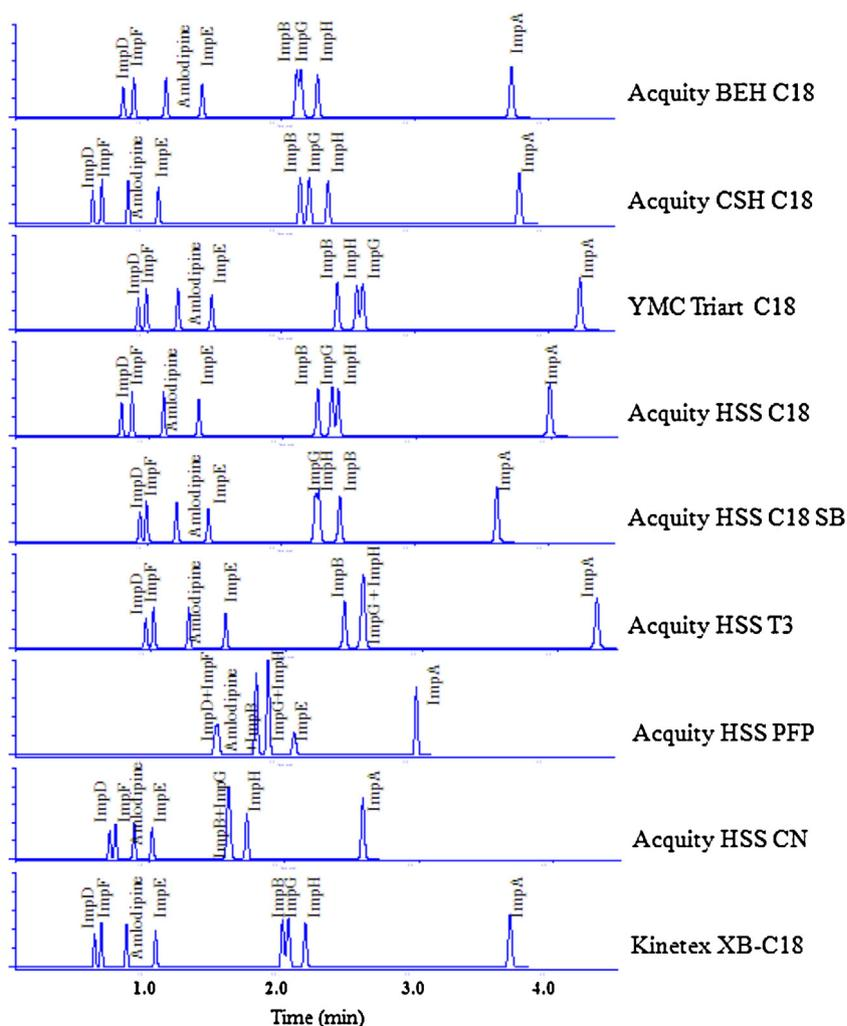
**Fig. 2.** Column selectivity comparison. Chromatographic parameters under the conditions  $t_G = 6$  min (from 30%B to 90%B),  $T = 30^\circ\text{C}$ ,  $\text{pH} = 2.5$ , for other conditions see Section 3.
