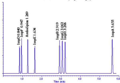
Fig. 7.4.a Predicted chromatogram on Acquity HSS C18 column,  $R_{s,crit}=2.45$  (ImpB-ImpG)
