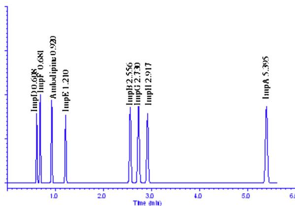
Fig. 7.9.a Predicted chromatogram on Kinetex XB-C18 column,  $R_{s,crit} = 2.18$  (ImpD–ImpF)
