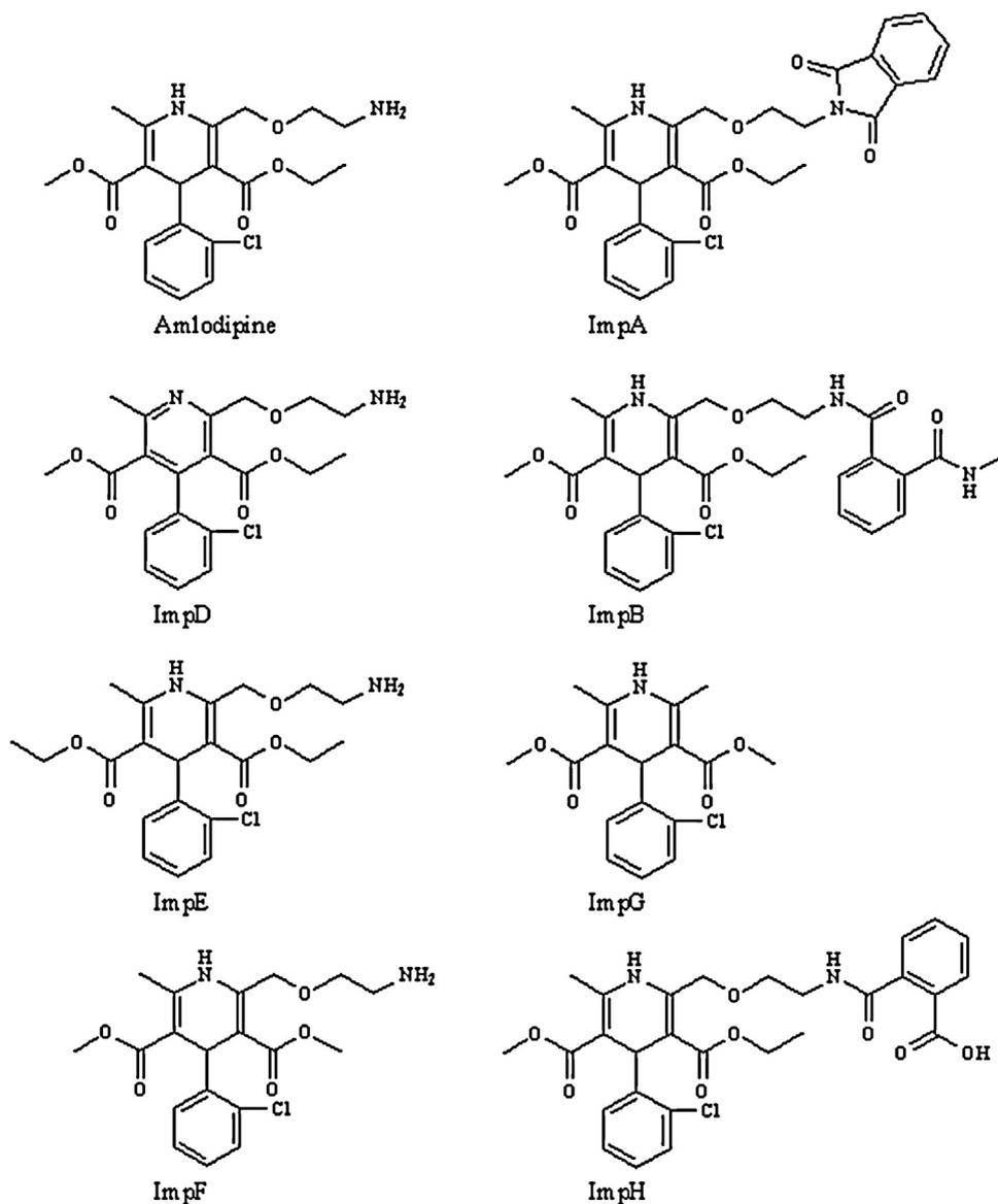
**Fig. 4.** Structure of amlodipine and its impurities. Amlodipine, ImpD, ImpE and ImpF contain free amino groups. ImpH contains free carboxylic group. There is a movement of ImpH with increasing pH to shorter retention times, which is of strong influence on the elution order. The basic groups have at the low pH rather limited influence.
