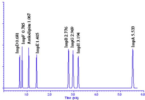
Fig. 7.2.a Predicted chromatogram on Acquity CSH C18 column,  $R_{s,crit}=3.06$  (ImpD-ImpF)
