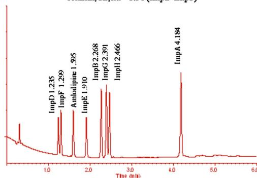
Fig. 7.7.b Experimental chromatogram on Acquity HSS PFP column,  $R_{s,crit}=1.51$  (ImpD-ImpF)
