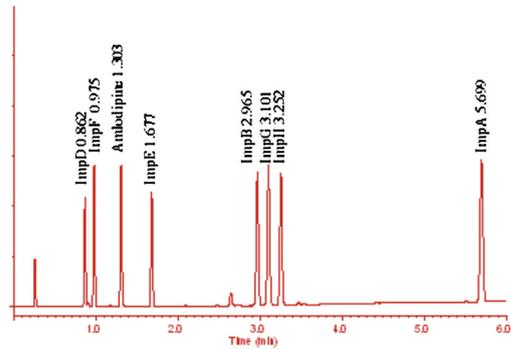
Fig. 7.4.b Experimental chromatogram on Acquity HSS C18 column,  $R_{s,crit}=2.63$  (ImpB-ImpG)
