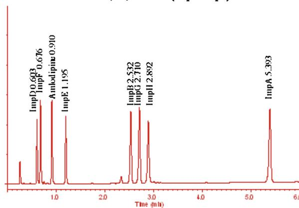
Fig. 7.9.b Experimental chromatogram on Kinetex XB-C18 column,  $R_{s,crit} = 2.33$  (ImpD–ImpF)
