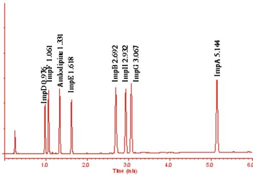
Fig. 7.3.b Experimental chromatogram on YMC Triart C18 column,  $R_{s,crit}=2.36$  (ImpD-ImpF)
