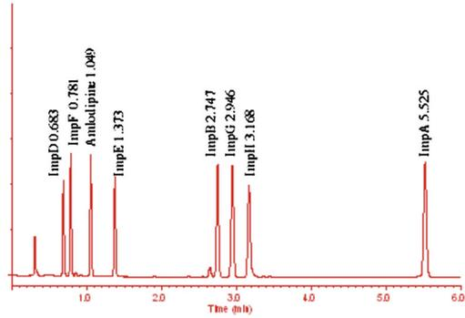
Fig. 7.2.b Experimental chromatogram on Acquity CSH C18 column,  $R_{s,crit}=2.91$  (ImpD-ImpF)
