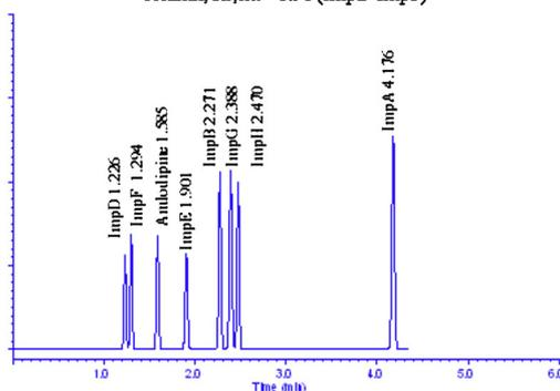
Fig. 7.7.a Predicted chromatogram on Acquity HSS PFP column,  $R_{s,crit}=1.58$  (ImpD-ImpF)
