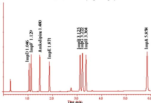
Fig. 7.6.b Experimental chromatogram on Acquity HSS T3 column,  $R_{s,crit}=1.73$  (ImpB-ImpG)
