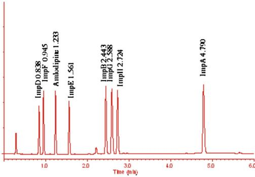
Fig. 7.1.b Experimental chromatogram on Acquity BEH C18 column,  $R_{s,crit}=2.92$  (ImpD-ImpF)
