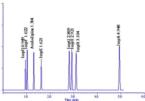
Fig. 7.5.a Predicted chromatogram on Acquity HSS C18 SB column,  $R_{s,crit}=2.01$  (ImpD-ImpF)
