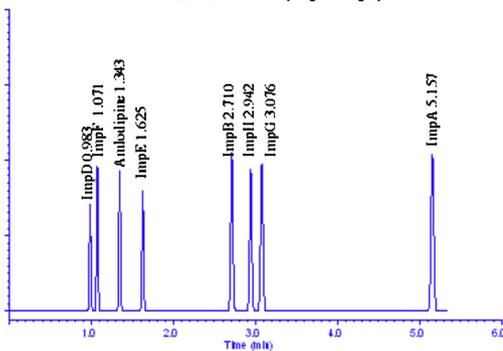
Fig. 7.3.a Predicted chromatogram on YMC Triart C18 column,  $R_{s,crit}=2.46$  (ImpD-ImpF)
