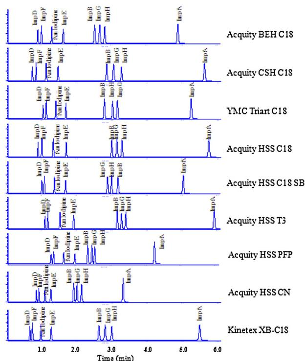
**Fig. 8.** The best separation on each column (experimental conditions see Section 3). Comparison of the 9 different columns after evaluating the best separation working point for each column. The selectivities are comparable and all peaks are baseline separated. The best robustness is provided with the CSH C18 column.
