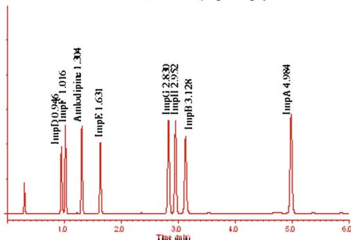
Fig. 7.5.b Experimental chromatogram on Acquity HSS C18 SB column,  $R_{s,crit}=1.91$  (ImpD-ImpF)
