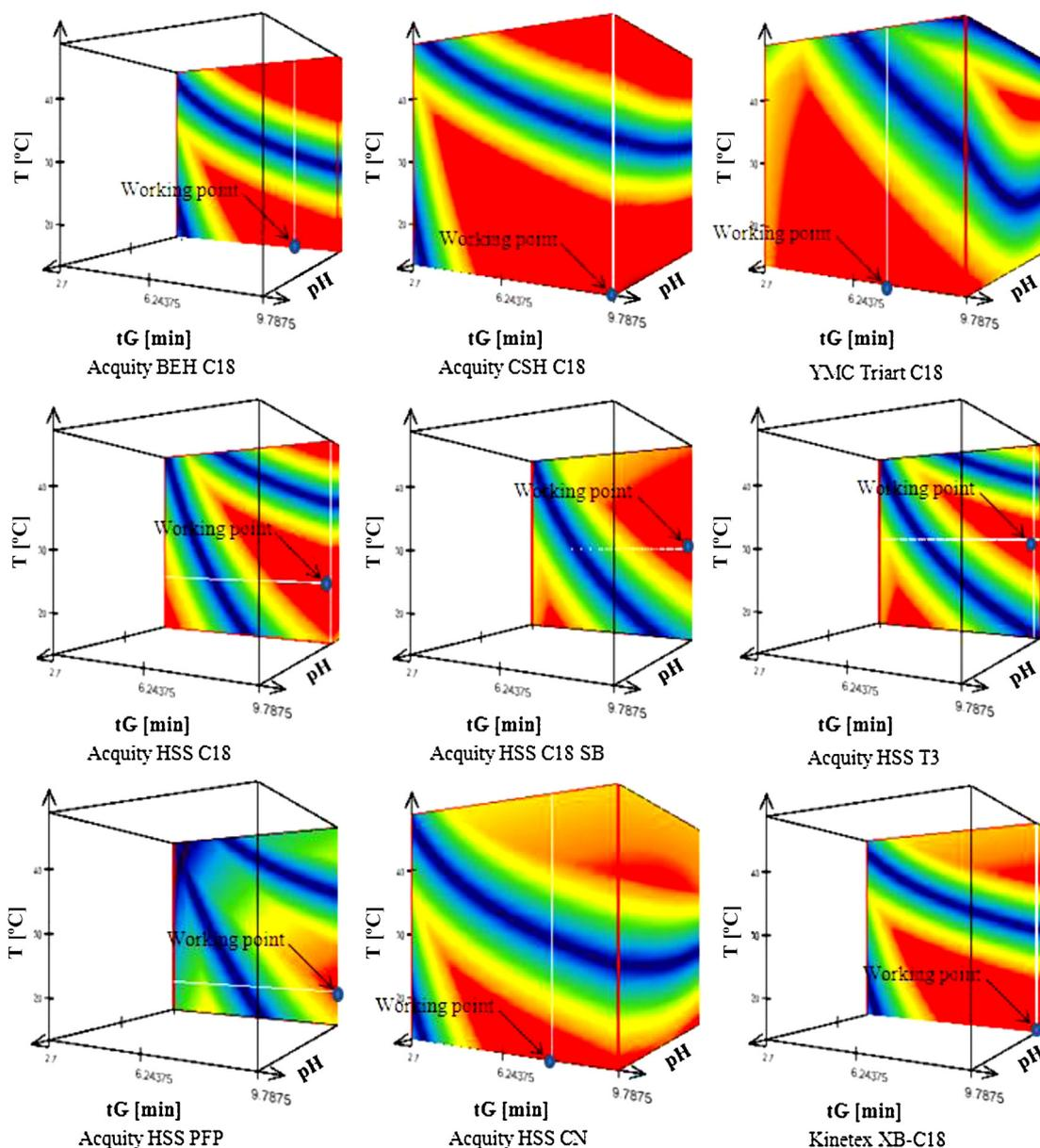
**Fig. 6.** Three-dimensional tG-T-pH models (cubes) on sub-2- $\mu\text{m}$  silica particle showing the best separations at the “Working points”. Note that although the working points are all at different positions, but we have in each cases a sufficient baseline separation. Red colours mean “baseline separation” ( $R_{s,crit} > 1.5$ ), blue colours indicate coelution ( $R_{s,crit} > 0$ ) of some peak pairs (experimental conditions see Section 3).
