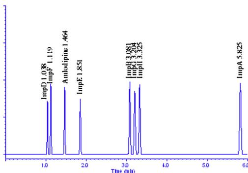
Fig. 7.6.a Predicted chromatogram on Acquity HSS T3 column,  $R_{s,crit}=2.17$  (ImpB-ImpG)
