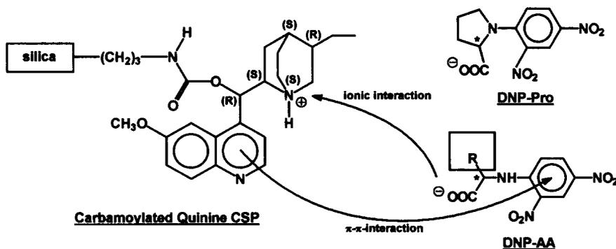
Fig. 1. Structure of the chiral stationary phase (CSP) as well as of the analytes (see also Table 1) and proposed sites of specific intermolecular interaction between the selector (SO) and the selectand (SA).
