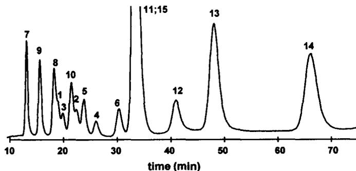
Fig. 3. Chromatogram at optimized experimental and isocratic conditions. (Mobile phase: 110 mM ammonium acetate-(ACN-THF, 99:1), (55:45, v/v); pH<sub>a</sub> 5.5; T=25°C; peak annotation see Table 1). The given molarity value refers to that of the final mixture.
