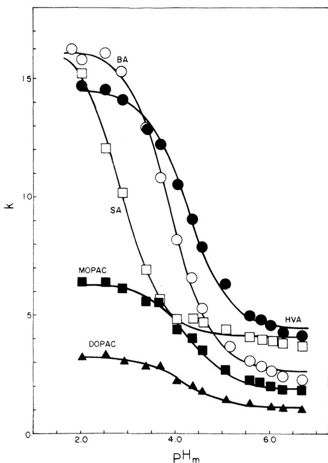
**Figure 6.** Plots of the capacity factor vs. the pH of the eluent for monoprotic acids
