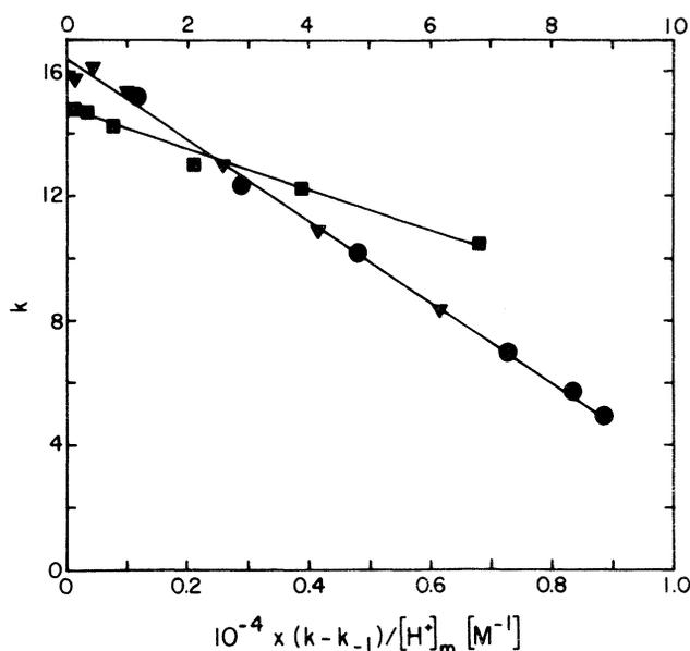
**Figure 7.** Plot according to Equation 23 to estimate the parameters which govern the pH dependence of the capacity factor of weak monoprotic acids
