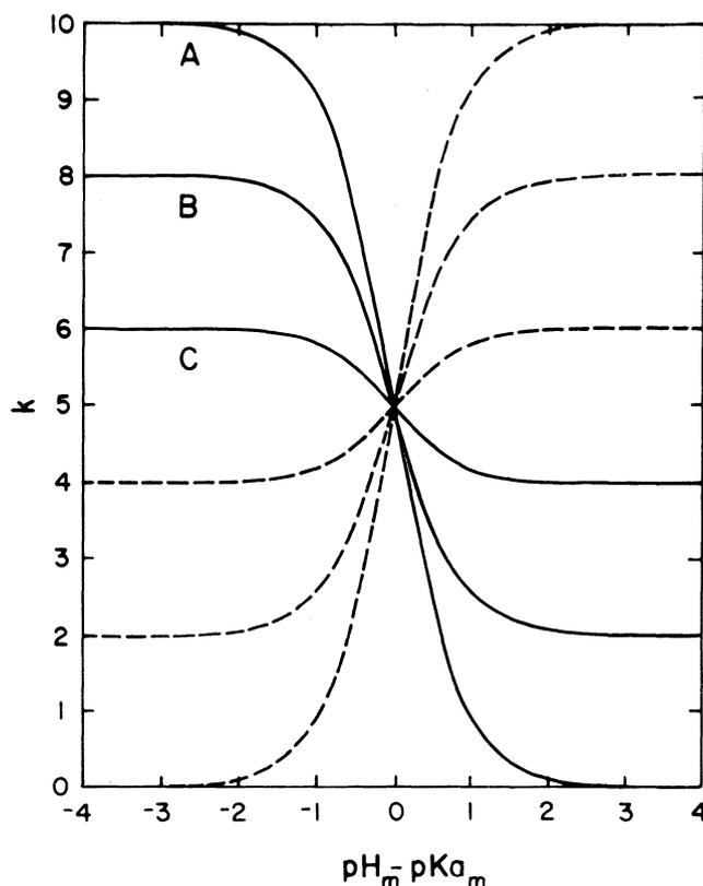
**Figure 5.** Plots of the capacity factor of weak monoprotic acids (solid lines) and bases (broken lines) vs.  $pH_m - pK_{a_m}$
